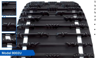
This utility track uses a modified version of the tried-andtested RipSaw design for improved traction in soft snow. The durable, full lug design provides excellent traction and features a 1.25" lug height, a popular upgrade for utility vehicles fitted with a 1" lug track for mile after mile of dependable use.
