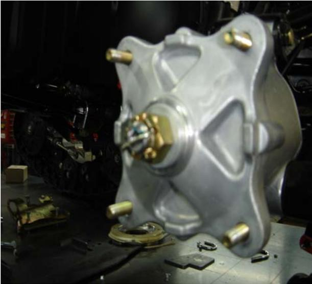
\*3. Put the hub spacer on the ATV hub.
