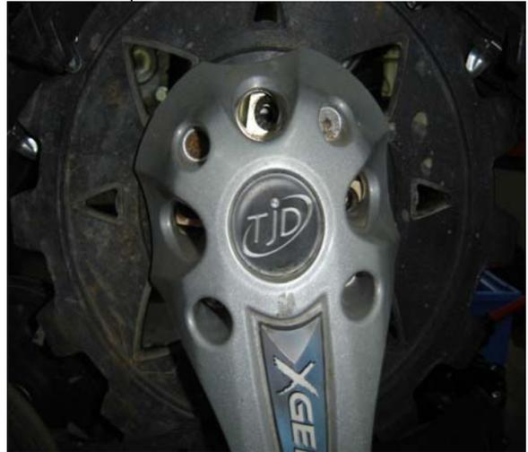
6. Position the sprocket of the XGEN assembly to allow the sprocket to fully engage into the hub adaptor.
