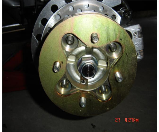
\*2. Put the hub spacer on the ATV hub.
