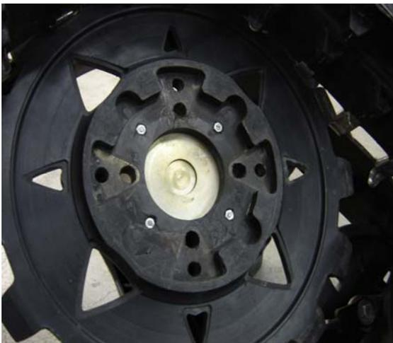
8. Bolt the XGEN assembly by the front side to the hub adaptor with the bolts provided with the hub adaptor. Apply threadlocker (Loctite) on the bolts.
