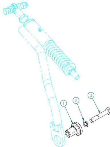
Remove the bolt and bushing spacers at the end of the rod. Then attach the stabilization rod to the adapter plate, making sure that the bushings are placed between the spacers and the rod support. If your stabilization rod support has three (3) positioning holes, use the central hole.
