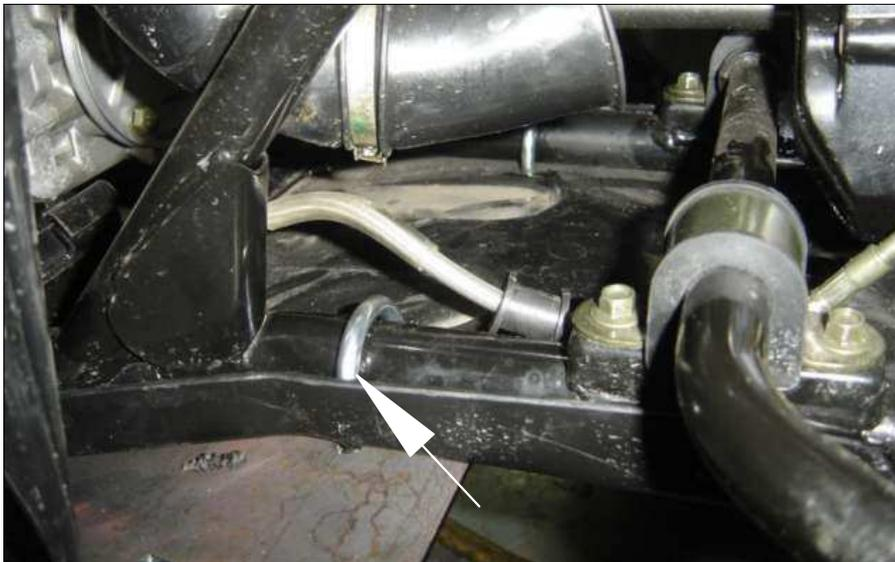
Install the U bolts on the frame as shown.
