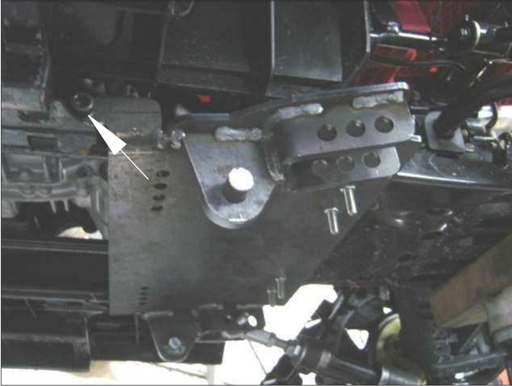
Remove the bolts in place. Install the part 03PA-277 and then reinstall the bolts that comes with the kit (as shown above).
