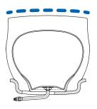
Camso CMP 576 compactor tire features robust tread construction with breakers designed to limit tread crowning. This helps **promote even tread wear** and reduced ground pressure.
