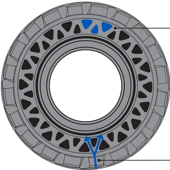
Deep, alternating triangular aperture holes minimize weight and stress on machine components
