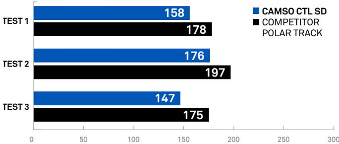
Throughout the entire tests, Camso's **braking distance on ice is 13% lower than competitor** offering a better handling and lower slippage
