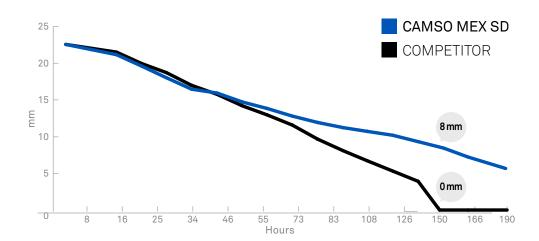
In this test, we clearly see that the competitor track tread compound was wearing faster versus Camso. Maintaining more rubber around the carcass offers more protection and translates in longer service life. The end result is: Camso MEX SD
