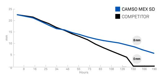
In this test, we clearly see that the competitor track tread compound was wearing faster versus Camso. Maintaining more rubber around the carcass offers more protection and translates in longer service life. The end result is: **Camso MEX SD** offers 20% more service life.
