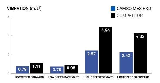
Throughout the entire test, the **vibration level was 42% lower with the Camso tracks** than the OEM quality track regardless the speed and the direction.
