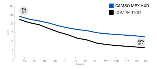
Camso tracks are designed with much thicker tread than most OEM tracks. Maintaining more rubber around the carcass offers more protection on carcass puncture and edge cutting. This all translates in longer service life and less downtime. The end result of this test is: Camso MEX HXD offers 30% more service life.
