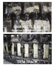
After 196 hours of test, the competitor tracks failed versus Camso, whose tread bar were in good condition all around the track.
