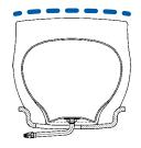
Camso CMP 576 compactor tire features robust tread construction with breakers designed to limit tread crowning. This helps **promote even tread wear** and reduced ground pressure.
