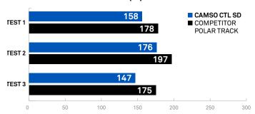
Throughout the entire tests, Camso's **braking distance on ice is 13% lower than competitor** offering a better handling and lower slippage
