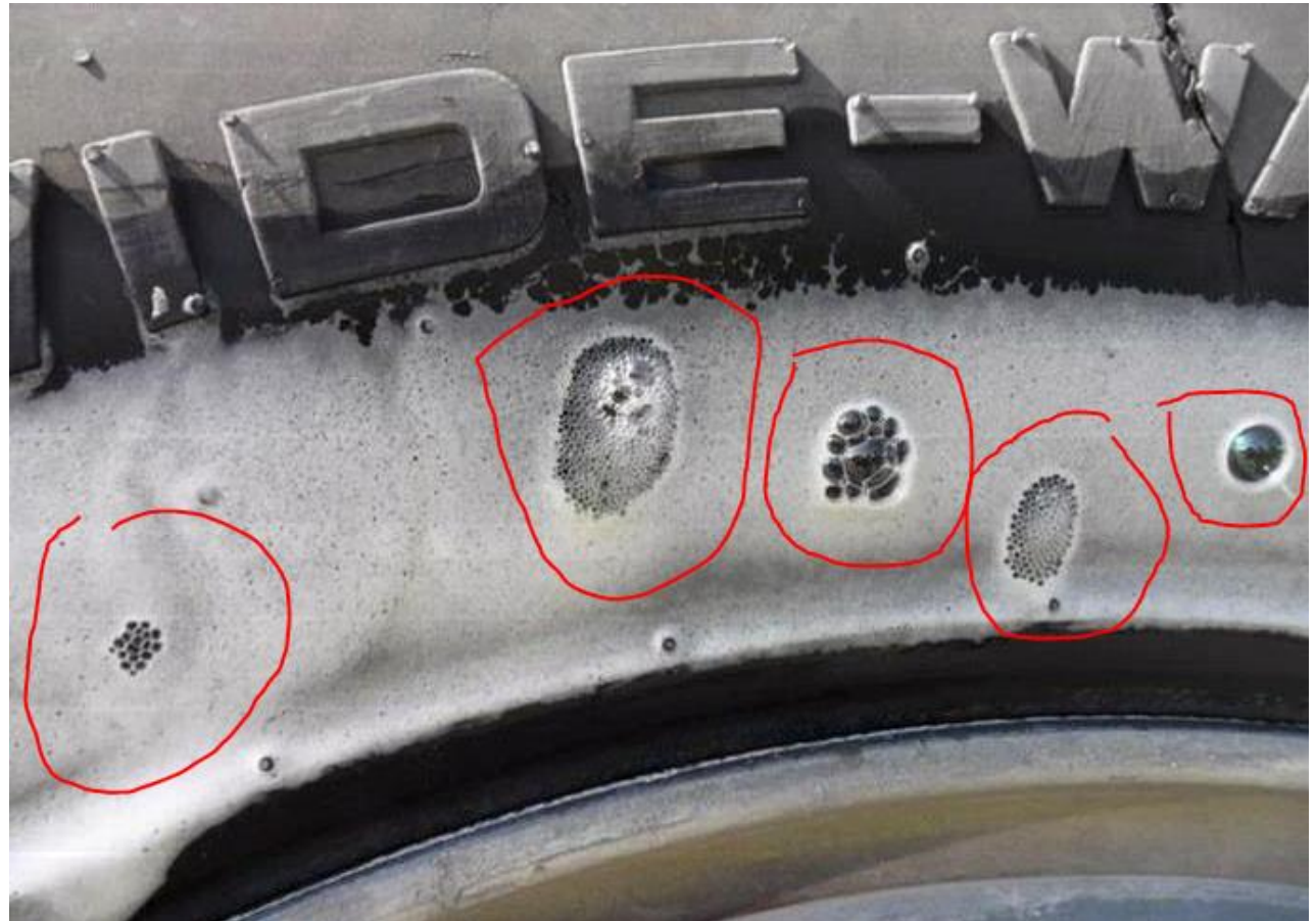
Air leakage shown by, adding soapy water to the tire's sidewall
