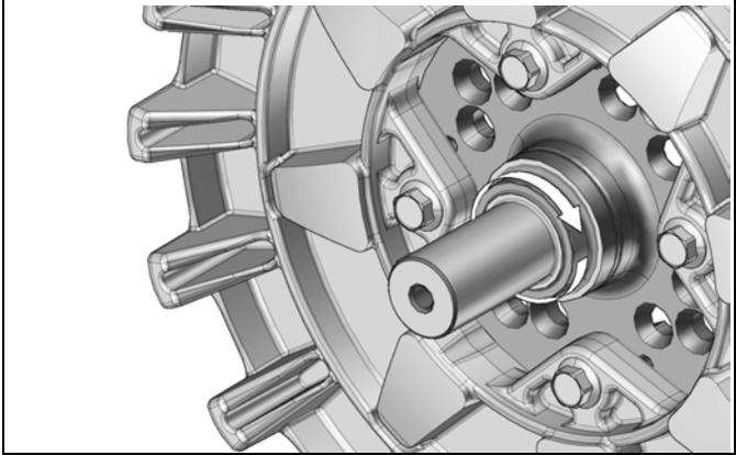
*NOTE: Replace Speed Sleeve immediately if defective.*
