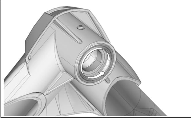
**IMPORTANT:** The hub seal must be installed flush with the hub face.
