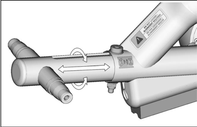
*NOTE: Application of lubricant on the tensioner tubing prevents corrosion inside the frame's tube. Lubrication allows the tensioner to move freely when adjusting the track's tension.*
