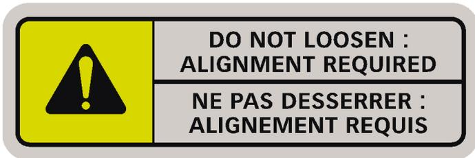
**TENSIONER BOLT WARNING** - If track tension adjustment is required, do not loosen the tensioner assembly bolt under any circumstance. The bolt is used to assemble and align the tensioner with the frame. Tensioner re-alignment is necessary if this bolt is loosened.
