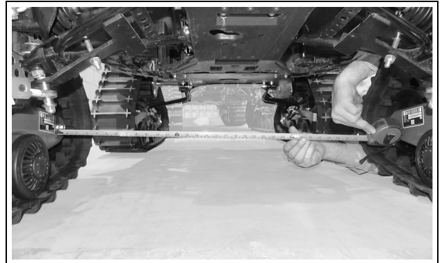
Figure 22 (Distance inside front frames - rear end)
