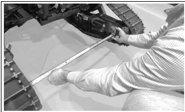
Figure 20 (Distance inside front frames - front end)
