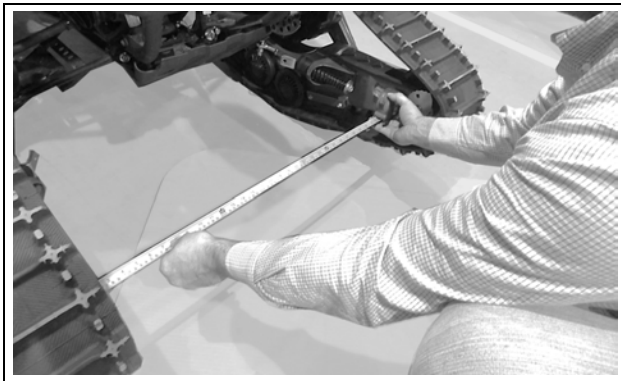
Figure 20 (Distance inside front frames - front end)
