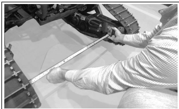
Figure 19 (Distance inside front frames - front end)
