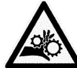
**Moving Parts** - Hands or fingers caught between moving parts of the equipment present a danger to life or limb. Turn motor off before servicing Conversion System.
