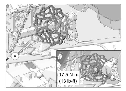
**IMPORTANT**: Perform the steps described above for all 6 Brake Rotor assembly bolts.
